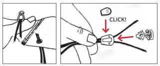
Take the loose ends of your lace and thread them from the outside through the eyelet on the other side of the gaiter. Attach the trimmer (2) as shown. First slide the housing, then put the spring in the housing and close everything with the cover. The closing can possibly just be done with a little force.
